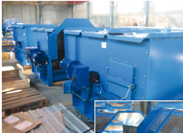
Assemblies completed at work shop ensure trouble free start-up and good belt tracking.
